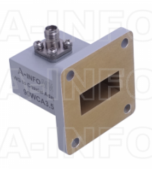
90WCA3.5 Right Angle Rectangular Waveguide to Coaxial Adapter 8.2-12.4GHz WR90 to 3.5mm Female
